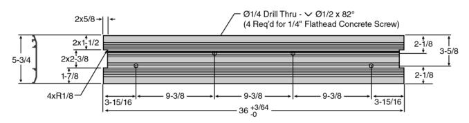
For anchorage to the concrete floor, thresholds shall be produced with pre-punched, countersunk holes to accept 1/4" diameter concrete sleeve anchors (provided by EXPI-DOOR). Three-foot single door system thresholds shall consist of four (4) countersunk bores, and shall be "staggered" across the length of the Threshold.
