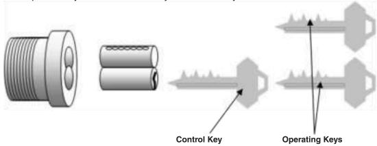
Figure-8 S.F.I.C. Cylinder Core in Falcon "A" keyway (comparable to BEST's most common keyway) - Used for cylindrical locks and key-in-lever exit device trim.
